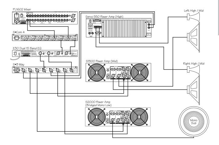
In this example, the S•com 4 is inserted after the mixer and before the graphic equalizer, thereby compressing the full range signal from the mixer.
