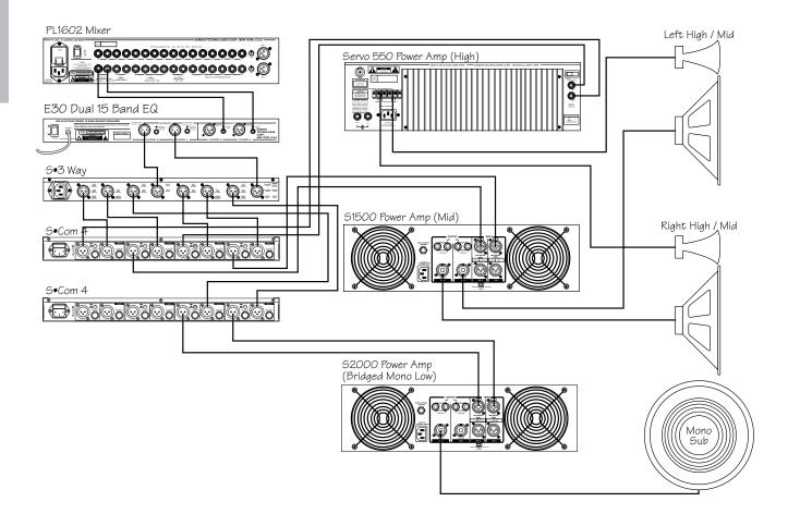
In this example, two S•com 4's are inserted after the mixer, equalizer and crossover, thereby providing individual compression on the low, mid and high frequencies.
